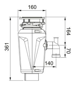
Elite Slimline 50 food waste disposer, 1/2 HP, Continuous Feed, High Torque Dual Magnetic Motor, Motor Speed 2600 RPM. 10 Year Guarantee on all Franke WDUs.
