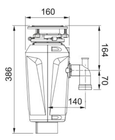
Elite Slimline 75 food waste disposer, 3/4 HP, Continuous Feed, High Torque Dual Magnetic Motor, Motor Speed 2700 RPM. 10 Year Guarantee on all Franke WDUs.
