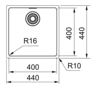
MRX 110-40 440x440x180mm, with overflow hole, with basket strainer waste 3 1/2" semi-integrated and overflow set, no drainer, no tap hole, packed in single box
