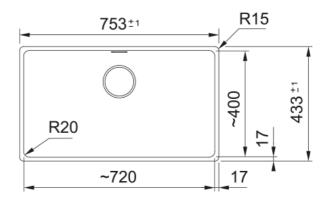
The Franke Maris MRG 110-72 is manufactured from an exceptionally tough material, highly resistant to burns, dents, chips and stains. Pioneered by Franke, it's a unique material with a subtle sheen that is warm to the touch thanks to its close to 80% of quartz sand. The surface is finely textured ensuring high hygiene standards. - Undermount installation. -  $3\frac{1}{2}$ " semi-integrated waste with circular cover-plate and hygienic overflow. - 50 year guarantee on all Franke sinks.
